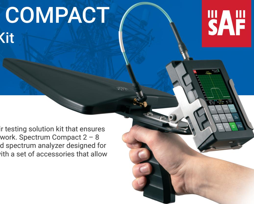
SAF Tehnika offers an over-the-air testing solution kit that ensures the stability of the 5G C-band network. Spectrum Compact 2 – 8 GHz is a rugged yet light handheld spectrum analyzer designed for RF testing in the field. It comes with a set of accessories that allow you to perform tests such as:
